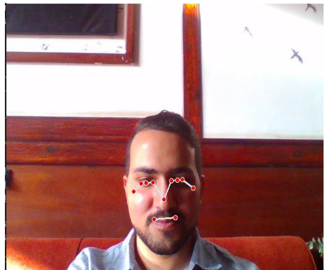
Fig.9. Head Pose Estimation Sample Result.
